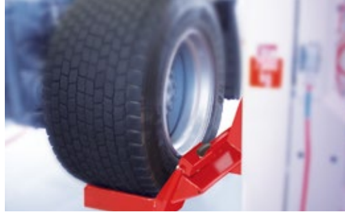
Lifting fork of 14" is well suited for super single tires.
