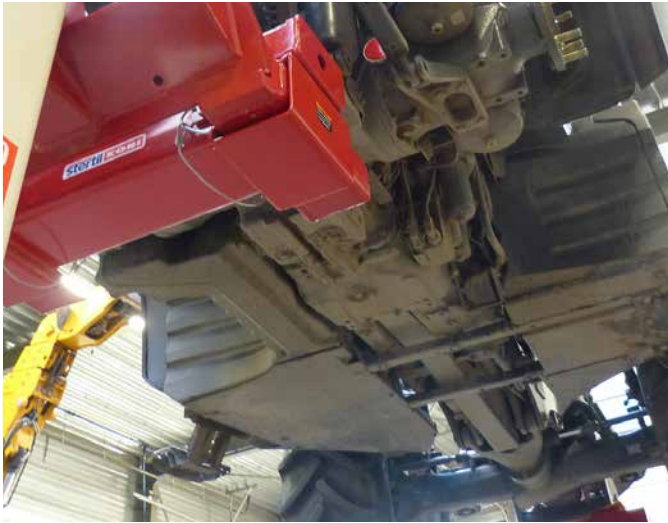
Special Pick-Up Adapters for wheel-free lifting.
