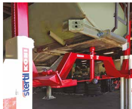
Traverse Kingpin Crossbeam for the safe and stable detachment and independent lifting of a trailer from the unit or cab.
