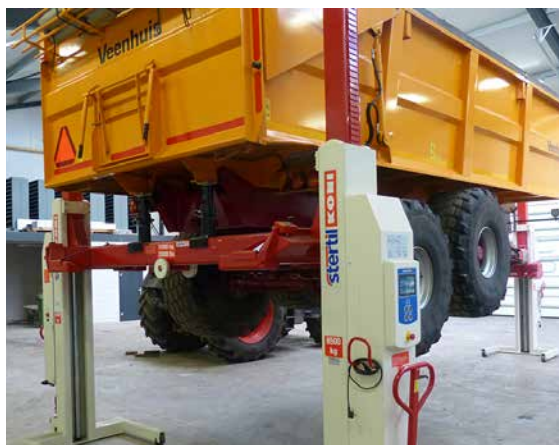
Low-Profile Crossbeam for more accessibility wheel-free maintenance.
